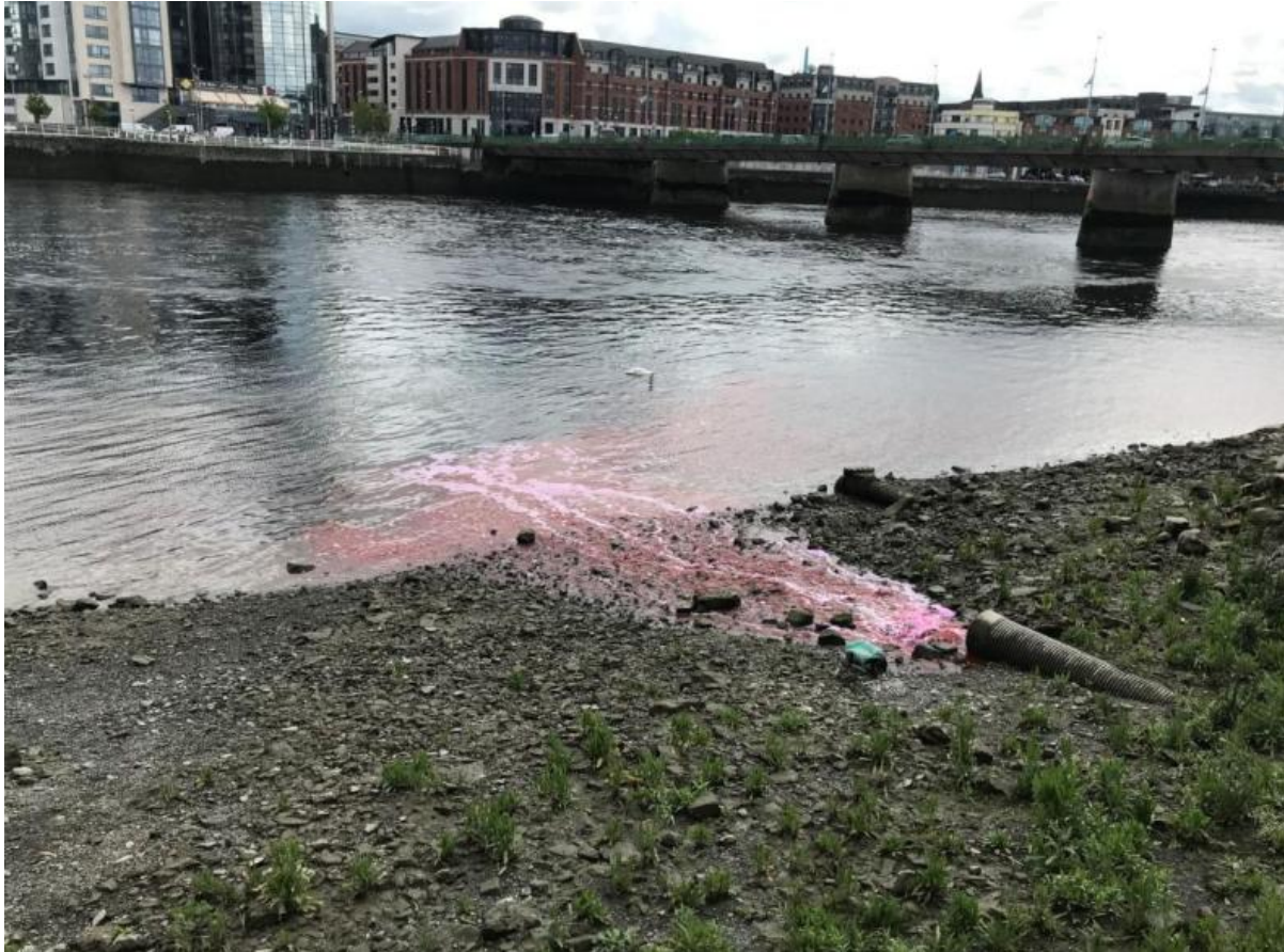
Figure 11-2 Discharge pipe at the River Shannon, during dye tracer testing (Source: Dye Tracer Survey Report (Irish Hydrodata Ltd., 2021))
